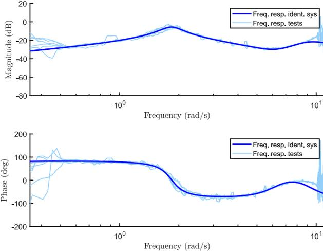
Fig. 4. Tests frequency responses and identified  $G_0$ .
