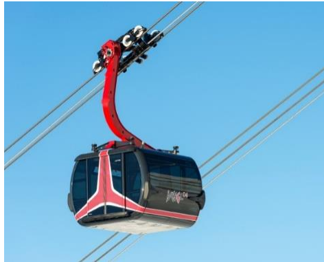
Figure 43-Picture of a bicable gondola with detachable grip vehicles with two carrying ropes (2)
