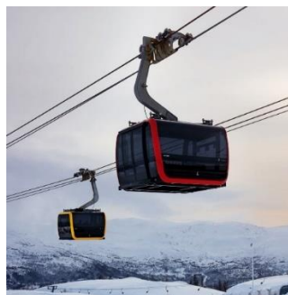
Figure 42-Picture of a bicable gondola with detachable grip vehicles with two carrying ropes
