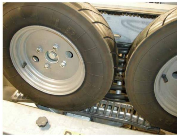
Figure 56-Detail on the tires mounted on the stations of traditional cable-car plant, that trigger the motion to the vehicle, allowing it to change its speed in the stations
