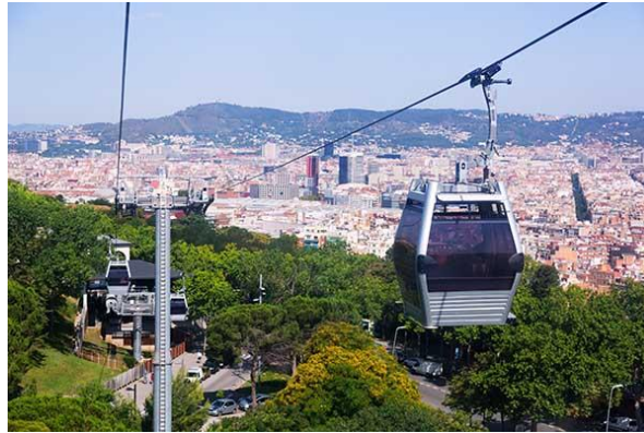
Figure 41-Picture of the urban traditional monocable gondola linking Barcelona with Montjuic, with emphasis on towers
