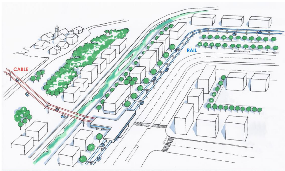
Figure 45-Sketch of an installation of a hybrid rope-motorized wheels system: the segment through rope, suitable to high sloped line, is indicated in red, while the segment in rail, allowing the definition of curves with small radius, is indicated in blue.
