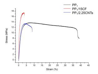
Figure 1. Tensile test curves referred to PP and its composites produced by FDM
