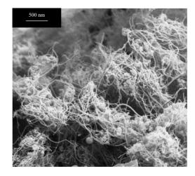
Figure 2. Carbon nanotubes located along laser tracks
