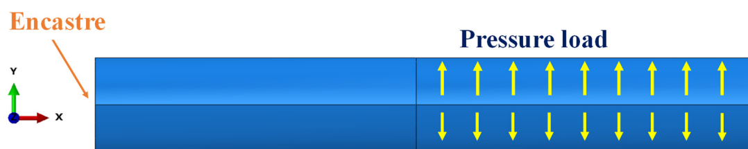
Figure 4. Boundary conditions on Abaqus/standard.
