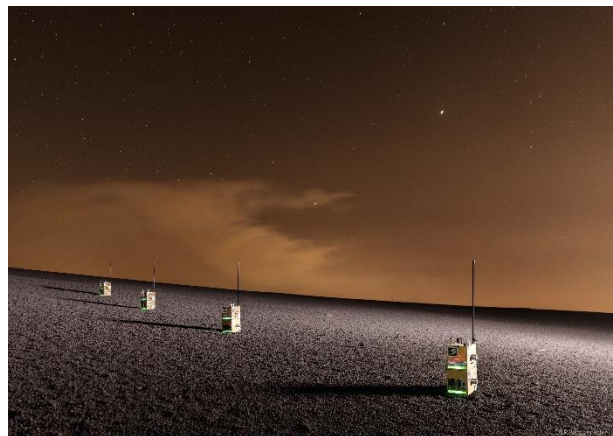
Fig. 18. RC-LOFAR deployed and in operation on Mount Etna during the night.
