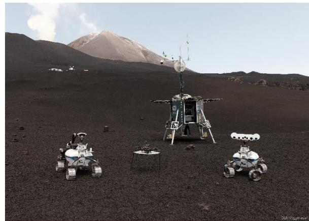
Fig. 2. Robotic Assets for ARCHES Demonstration Mission
