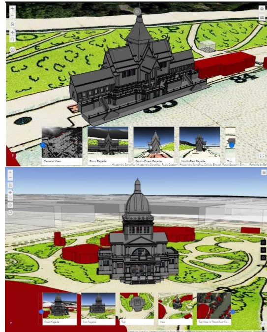
Figure 11. WebGIS application with integrated BIM model of the reconstructed Pavilion of Siam (up) and of City of Turin (down).
