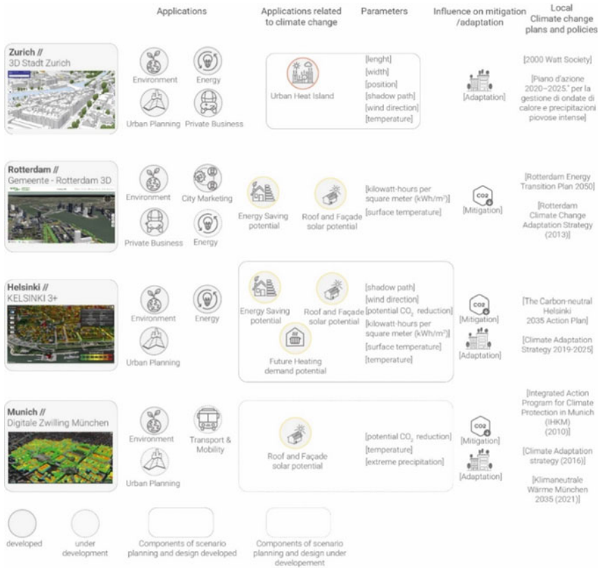
Fig. 55.2 Analysis of urban digital twin to support climate change scenario planning and design. Sources Stadt Zürich Geomatik, “3D-Stadtmodell” 2022. Accessed via https://web.stzh.ch/appl/3d/zuerichvirtuell/ ; Gemeente Rotterdam, “Rotterdam 3D” 2022. Accessed via https://www.3drotterdam.nl/#/ ; Helsinki 3D, “Energy and Climate Atlas” 2022. Accessed via https://kartta.hel.fi/3d/atlas/#/ ; Geoportal Muenchen, “Potenzialflächen Photovoltaik” 2022. Accessed via https://geoportal.muenchen.de/portal/energie/#/
