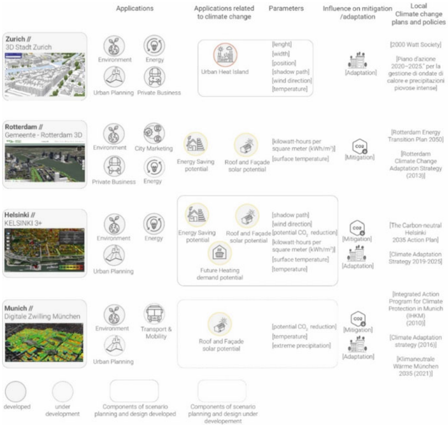
Fig. 55.2 Analysis of urban digital twin to support climate change scenario planning and design. Sources Stadt Zürich Geomatik, “3D-Stadtmodell” 2022. Accessed via https://web.stzh.ch/appl/3d/zuerschvirtuell/ ; Gemeente Rotterdam, “Rotterdam 3D” 2022. Accessed via https://www.3drottterdam.nl/#/ ; Helsinki 3D, “Energy and Climate Atlas” 2022. Accessed via https://kartta.hel.fi/3d/atlas/#/ ; Geoportal Muenchen, “Potenzialflächen Photovoltaik” 2022. Accessed via https://geportal.muenchen.de/portal/energie/#/
