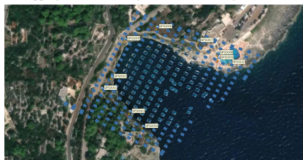
Figure 3. UAS nadir images acquisition scheme.
