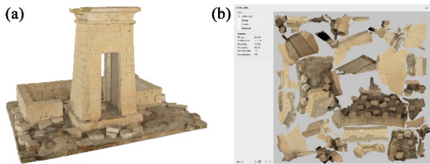
Figure 2. (a) Texture 3D model ('Dendur portal' wooden model); (b) UV map.
