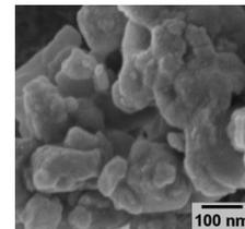
Figure 3. SEM image of LiNi<sub>0.8</sub>Mn<sub>0.1</sub>Co<sub>0.1</sub>O<sub>2</sub>
