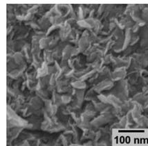
Figure 2. SEM image of Ni<sub>0.8</sub>Mn<sub>0.1</sub>Co<sub>0.1</sub>(OH)<sub>2</sub>
