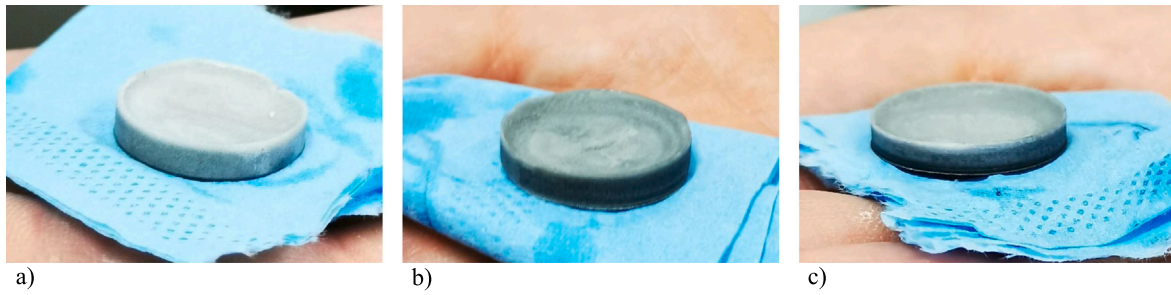
Fig. 3. Samples of PT15 additivated with (a) 0.132%, (b) 0.533% and (c) 1.11% in weight content of GNP15. In (b) and (c), the darker portion of the material at the bottom is due to the partial precipitation of the nanofillers.
