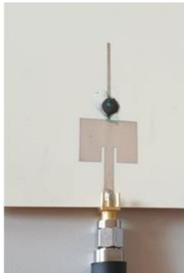
Figure 8. Sensor with drop of HRP.
