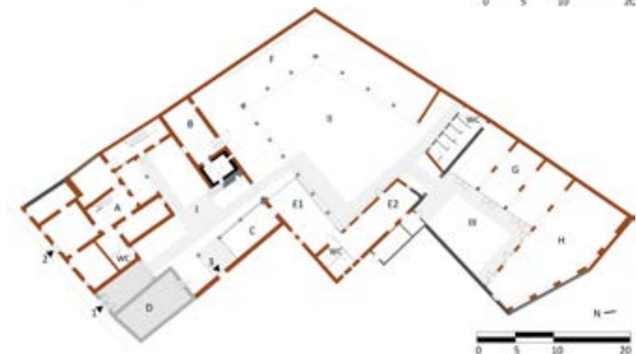
Figure 6: Project plan, ground floor. Courtyard I: A) exhibition rooms and tourist agency; B) storerooms; C) tasting rooms; D) Villa Fenu; 1) portal and entrance hall to the courtyard; 2) main entrance; 3) connection to Villa Fenu. Courtyard II: E1) cafeteria and E2) kitchens; F) exhibition area. Courtyard III: G) workshop and laboratories; H) conference room. Red: ladriri masonry; black: concrete; dark grey: stone masonry; grey: fired bricks and hollow bricks
