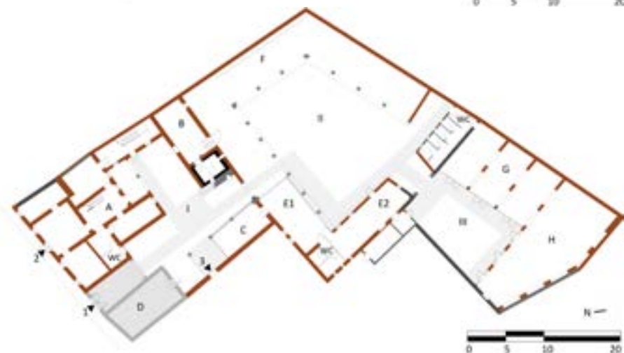
Figure 6: Project plan, ground floor. Courtyard I: A) exhibition rooms and tourist agency; B) storerooms; C) tasting rooms; D) Villa Fenu; 1) portal and entrance hall to the courtyard; 2) main entrance; 3) connection to Villa Fenu. Courtyard II: E1) cafeteria and E2) kitchens; F) exhibition area. Courtyard III: G) workshop and laboratories; H) conference room. Red: ladriri masonry; black: concrete; dark grey: stone masonry; grey: fired bricks and hollow bricks
