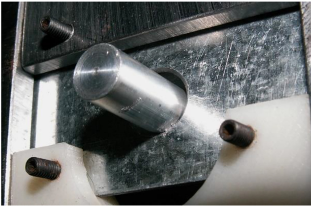
Fig. 3. Detail of the contact area between the AA2024 specimen and the sheet metal during the wear test.
