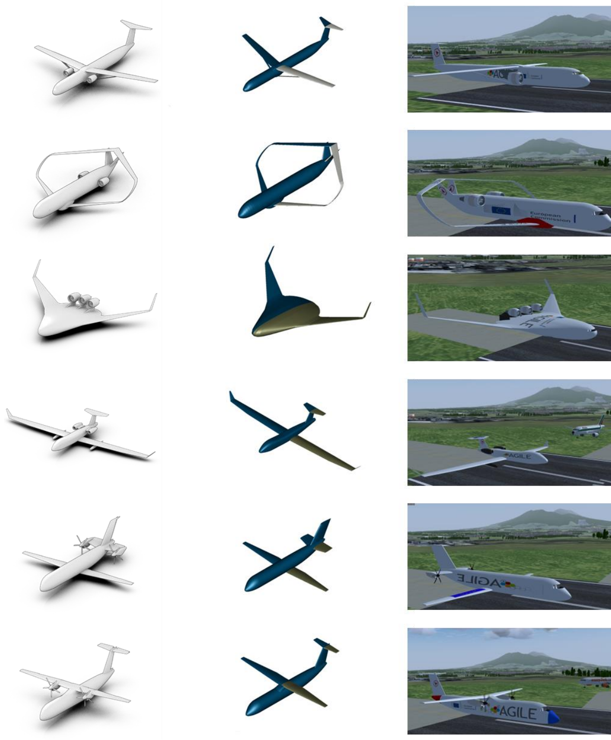
Fig. 46 AGILE Novel configurations (left) available in the database and corresponding CPACS models (middle) and FlightGear models (right).
