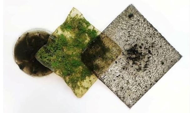
Figure 1: Samples of bioplastic sheets obtained using different concentrations of microalgae spirulina and musk. Author and credits: Selenia Marinelli.
