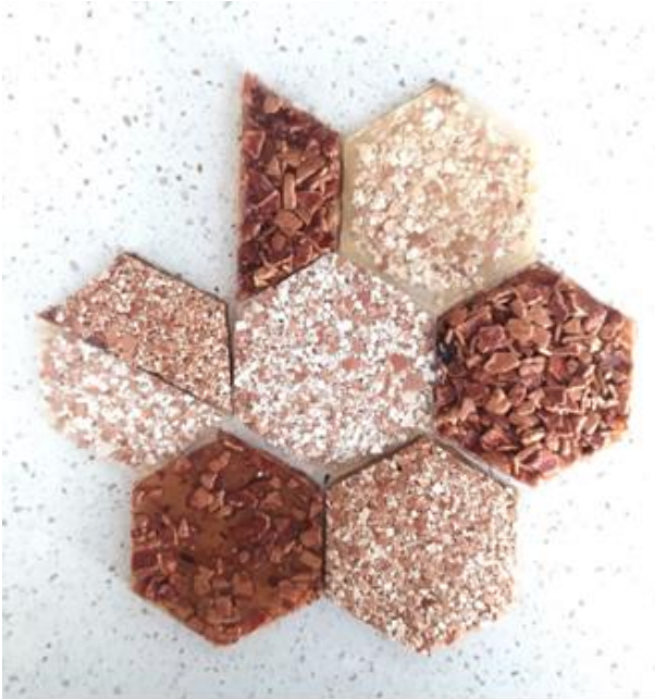
Figure 3: Bio-tiles made from different residues and biological, organic matter (eggshells, walnut shells). Author and credits: Selenia Marinelli.
