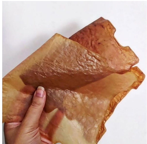
Figure 2: Bacterial cellulose sample grown from a SCOBY (symbiotic culture of bacteria and yeasts). The bacterial cellulose was dried after the fermentation process and it could be used as a vegan alternative to animal leather. Author and credits: Selenia Marinelli.
