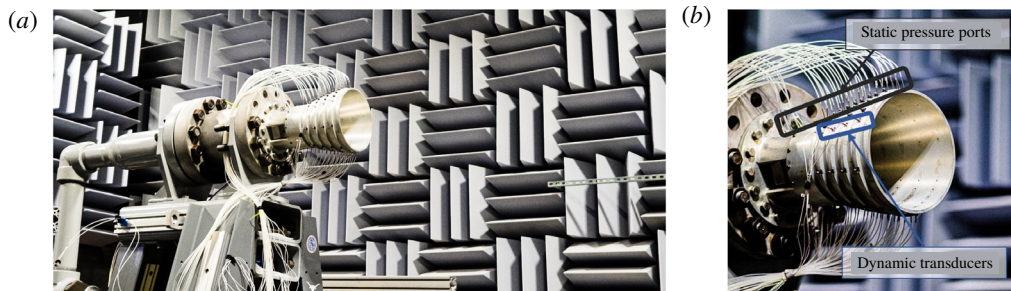
FIGURE 3. (a) Photo of the anechoic test environment at the University of Texas at Austin where the experiments were performed. (b) Photo of a nozzle installed on the test rig highlighting the tubing and wiring associated with the static and dynamic pressure ports.
