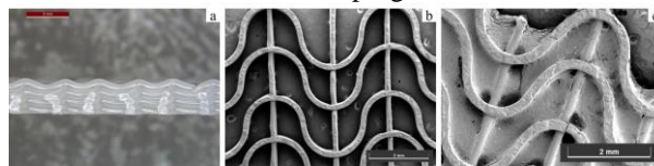
Fig.1 a) Optical and b) SEM images (40x) of PCL scaffold. c) SEM image of PCL/GelMA scaffold (37x).
