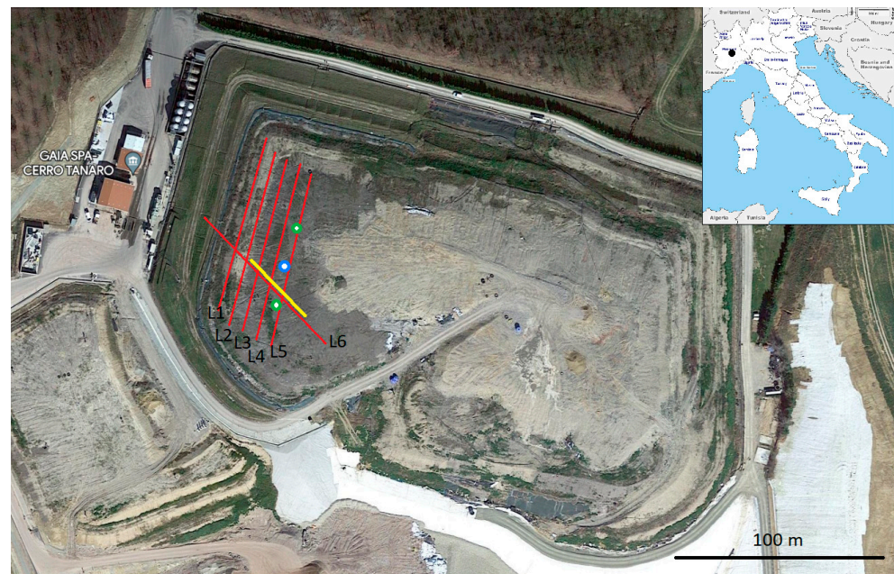
Figure 1. Test site with the position of the transects of the ERT on the landfill (L1–L6); the coordinate of the lower-left corner of the image is 44^{\circ}53'02\text{ N}-8^{\circ}22'7\text{ E} . The image is aligned south to north along the vertical direction. Red lines refer to the ERT lines of the preliminary characterization (48 electrodes, spacing 2 m): the labels of each line indicate the position of the first electrode of each section (relative coordinate of 0 m). The yellow line refers to the position of the ERT adopted for the infiltration test (48 electrodes, spacing 1 m); the first electrode is located at the south-east side. The blue circle refers to the injection well of the test of leachate recirculation; the green circle refers to the position of the borehole, which is addressed with electrodes and used for monitoring the leachate recirculation process within the landfill.
