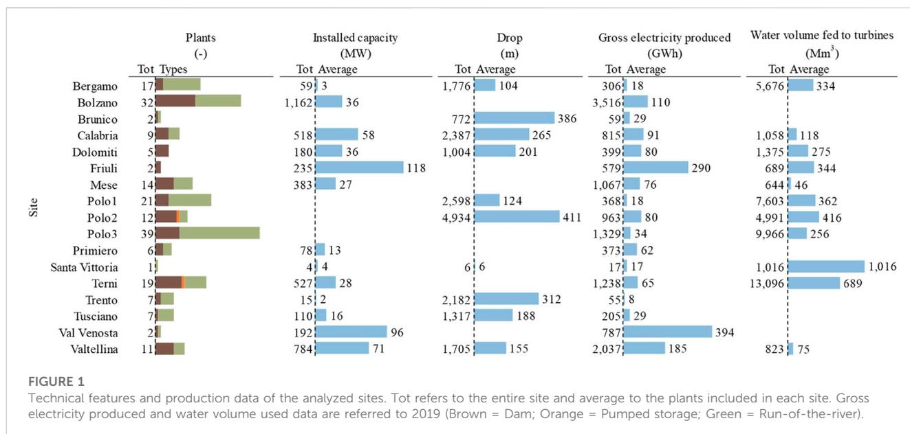
On average, each plant produced 68.5 GWh of gross electricity using 313 Mm<sup>3</sup> of water in 2019.
