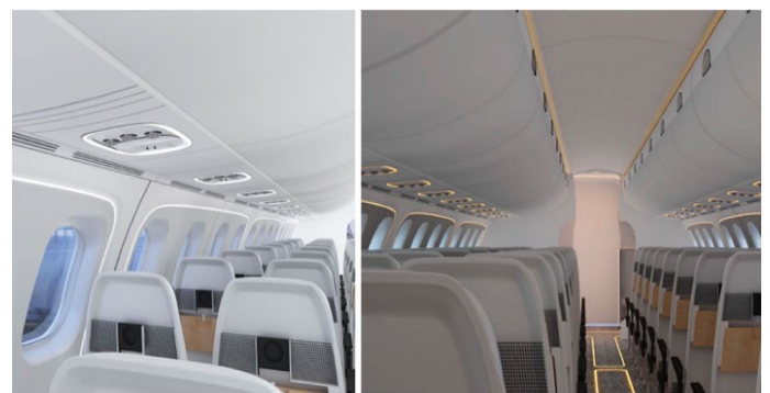
Fig. 10. The preparation of the CASTLE cabin (concept design in collaboration with Pininfarina) with white light LEDs and possible variation of intensity and color through RGB LEDs.
