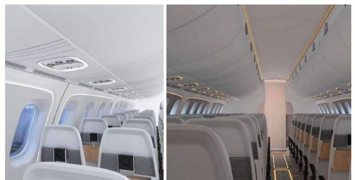
*Fig. 10. The preparation of the CASTLE cabin (concept design in collaboration with Pininfarina) with white light LEDs and possible variation of intensity and color through RGB LEDs.*
