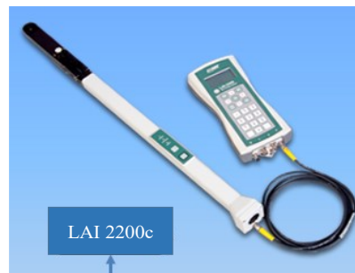
Figure 6. LAI-2200C PCA for LAI measurements.
