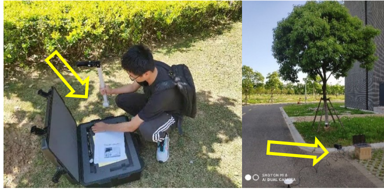
Figure 8. LAI measurements were obtained with an LAI-2200C PCA (left) and GNSS signal receiver (right).
