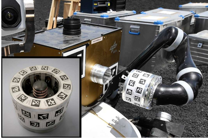
Figure 6: The ENVICON docking interface with retracted springs (lower left) and with extended springs about to dock to the payload box (right).
