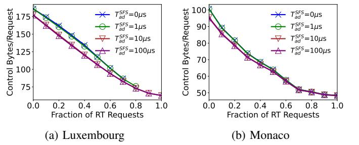
Fig. 2: Per-request signaling overhead due to DAPP-ECC.
