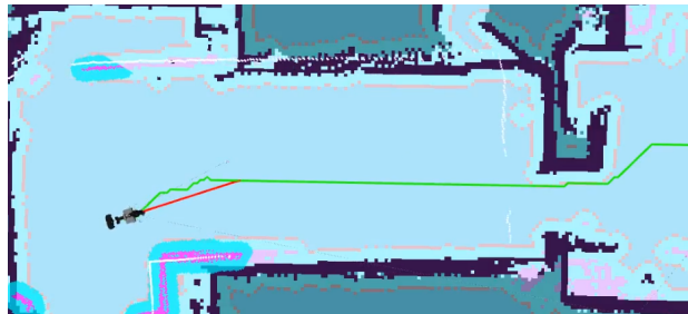
Fig. 2: Testing map visualization in rviz . Global path and local path plans are in green and red, respectively.
