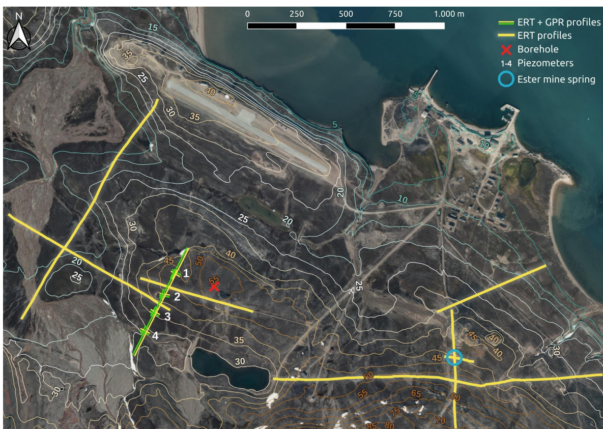
Fig. 1 – Map of the geophysical campaign carried out in Ny-Ålesund (Svalbard) in the summer of 2022. The ERT profiles are plotted in yellow and the GPR profiles in green. The investigated area on the west is the Bayelva river basin, while that on the east is the former mine. The piezometers are indicated with white numbers. The red cross is a recent borehole (48.5 m deep). The blue circle indicates the position of a spring (Haldorsen and Heim, 1999).
