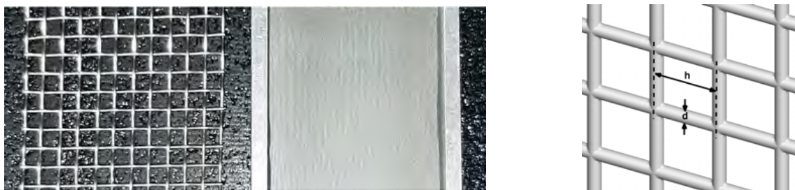
Fig. 4 Wire mesh samples considered in the study. Left: coarse wire mesh and fine wire mesh. Right: geometrical wire mesh parameters d and h .
