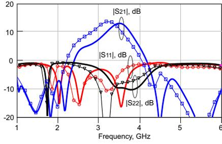
Fig. 3. Simulated (solid) and measured (symbols) scattering parameters.
