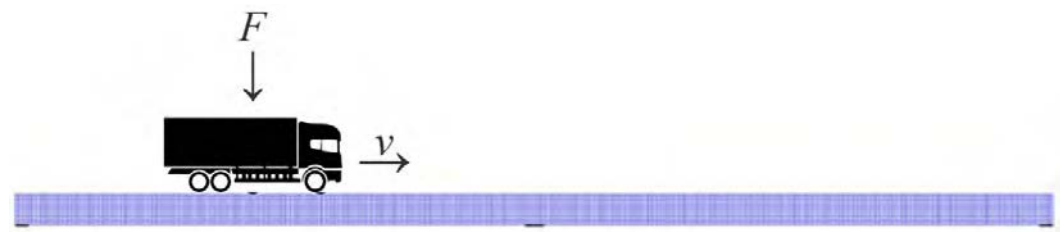
Figure 4. Loading in the form of a moving vertical force F with a constant speed v .
