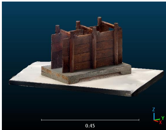
Figure 2. The digitization and virtual reconstruction of Curioni Model: the point cloud acquired by laser scanner.
