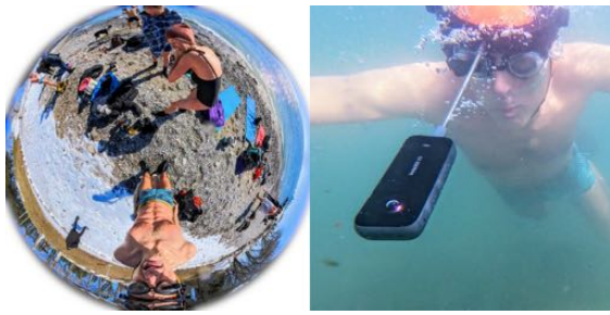
Figure 6. Experimental “Unicorn Vision” system functions as a “bird’s-eye-view” seeing aid for persons having a back injury, allowing a clear downwards-facing “foot first” view of the ground immediately beneath the wearer’s feet, to be streamed live to a “headup” display. Left: live video feed from camera. Right: experimental apparatus (underwater). Thanks to Dan Bowman + SwimOP for the underwater picture.
