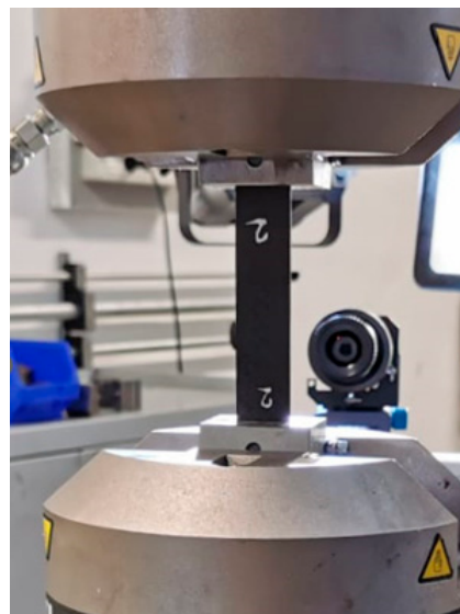
Figure 2. Tensile tests on composite laminates: testing configuration.
