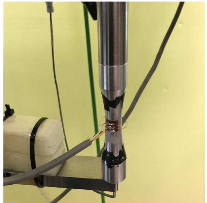
FIGURE 4 Specimen of 12 mm in diameter equipped with T-rosette strain gauge. [Colour figure can be viewed at wileyonlinelibrary.com ]
