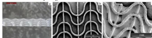
Figure 1. a) Optical and b) SEM images (40x) of PCL scaffold. c) SEM image of PCL/GelMA scaffold (37x).
