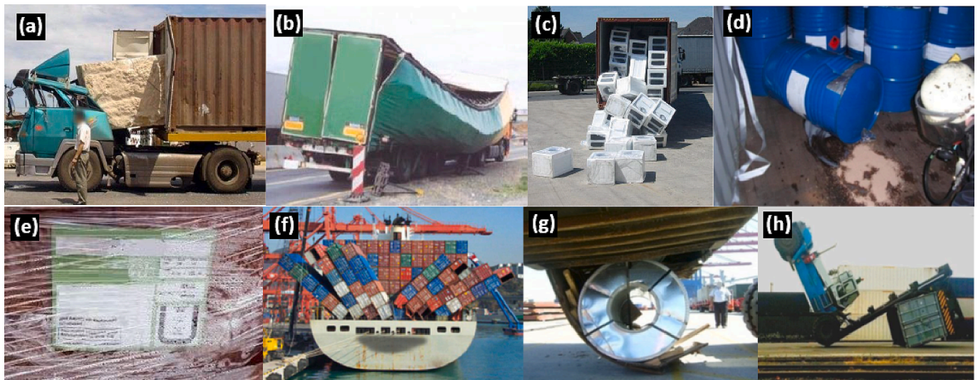
Fig. 1. Consequences of badly packed and secured cargo: lack of longitudinal securing (a); inadequate side wall strength (b); unsecured packages (c); spilled liquid dangerous goods (d); consequences of insufficient control of humidity, condensation damage (e); consequences of improper documentation and misdeclaration, stack failure (f); consequences of the use of unsuitable CTUs, overstressed floor (g); consequences of overloading of CTUs, tipped container handler (h). Source: CTU Code, informative material 1.
