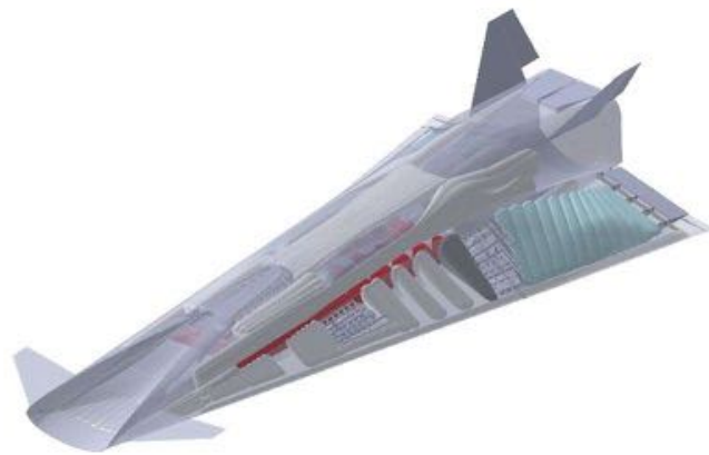
Figure 1. STRATOFly MR3 Vehicle layout with integrated systems.
