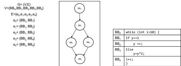
**FIGURE 1.** Sample code and program CFG example. The execution from basic block  $BB_1$  to  $BB_2$  or from  $BB_1$  to  $BB_3$  are legal, but a jump from  $BB_1$  to  $BB_4$  is illegal and called Control Flow Error (CFE).
