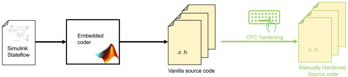
**FIGURE 2.** Indication, inside the model-based flow, indicating when the CFC is applied using high-level programming languages. The source code is obtained automatically via the Mathworks Embedded Coder from a Simulink semi-formal model, then the obtained source code is manually hardened.
