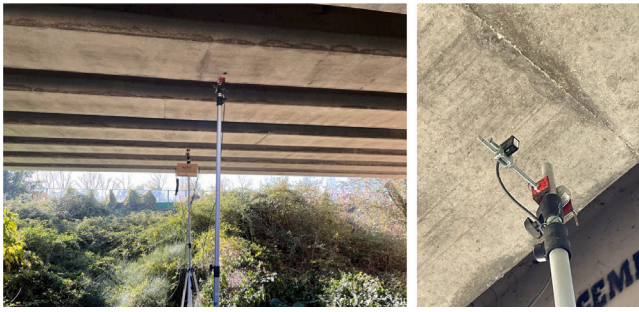
Fig. 12. View of the sensors layout and experimental setup in the Orte-Falconara bridge (1st case study) for the bridge deflection measurement using laser sensors under the train transit.
