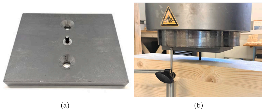
Fig. 5. Setup of specimen with height 540 mm in ZwickRoell Z1200-Steel plate used for Torx tests — Setup of Torx test.
