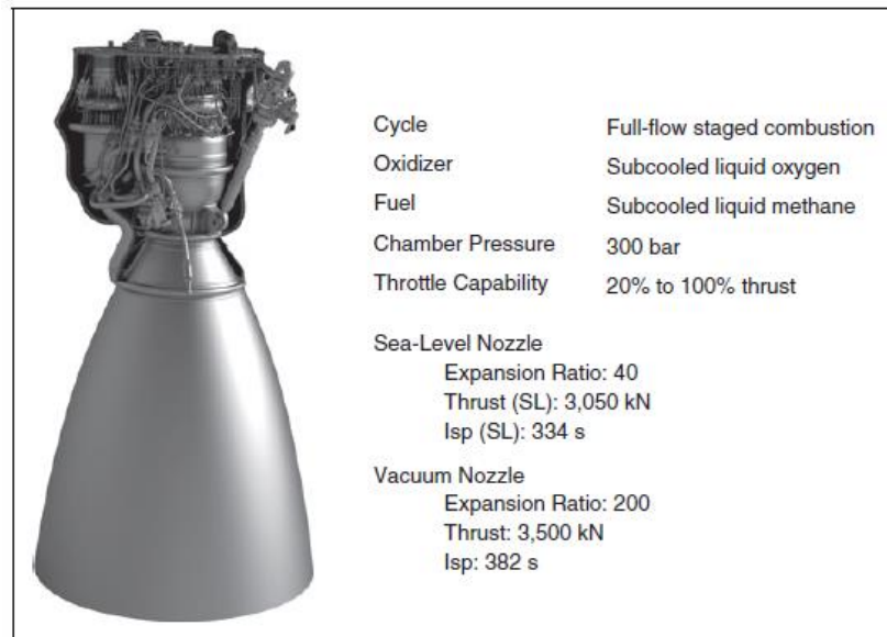
Fig 5. Key characteristics of the Raptor engine [2]
