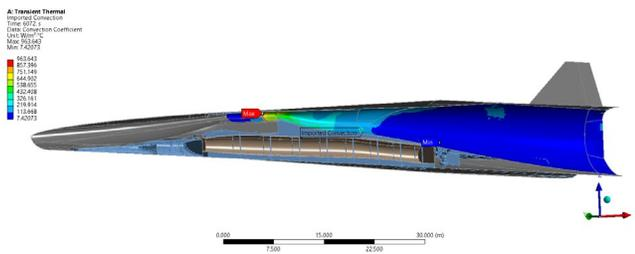
Fig. 23. Imported convection on internal combustion chamber surfaces.
