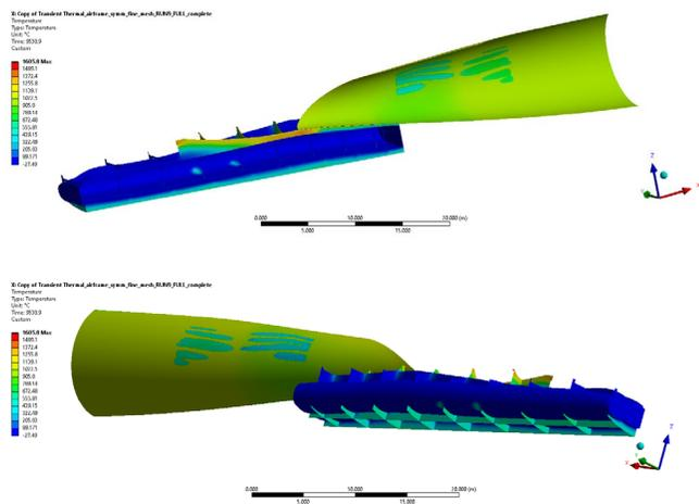
**Fig. 28. Temperature map at passenger cabin and surrounding stiffener box structure (a – internal view; b – external view): heat transfer mechanism.**
