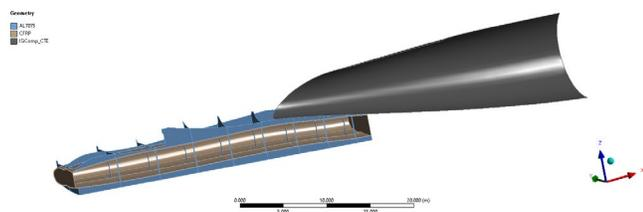
**Fig. 29. Passenger cabin, stiffener box, nozzle material distribution.**
