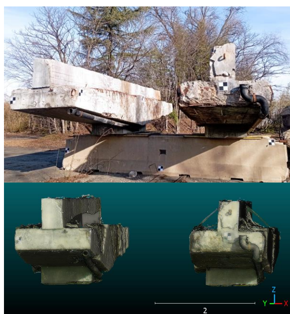
Figure 1. Up: photo of the studied beams. Bottom: TLS-generated point clouds of the studied beams.
