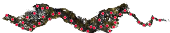
Figure 5. The top view of the point cloud generated by the BLK2GO system. In red are identified the waypoint.
