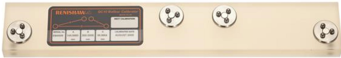
Fig. 6 Calibrated artefact (scale bar) used for the structured tests, to assess the instruments’ metrological performance in the shipbuilding context
