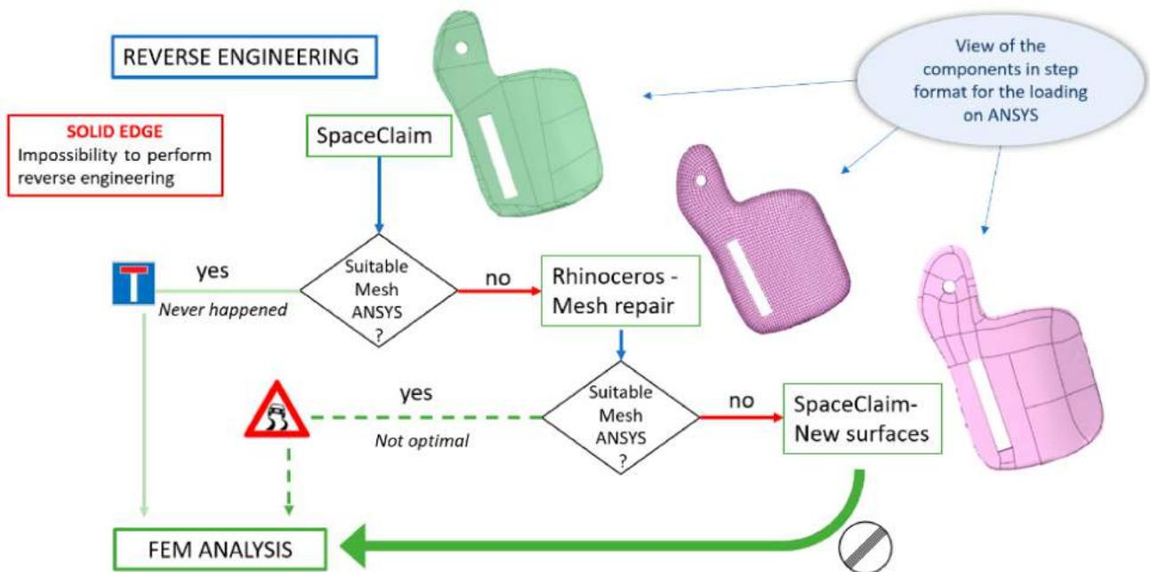
Figure 4. The final procedure for reverse engineering.
