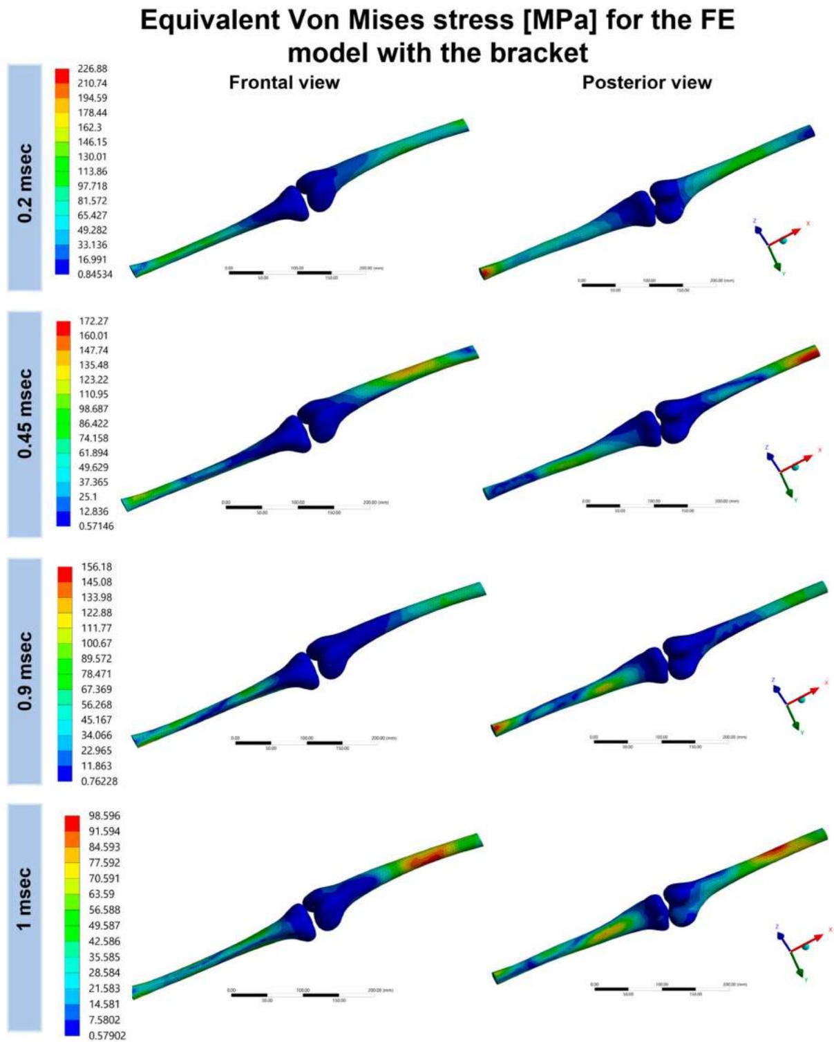
**Figure 8.** Equivalent Von Mises stress distribution in the bone component of the limb for the FE model with bracket.
