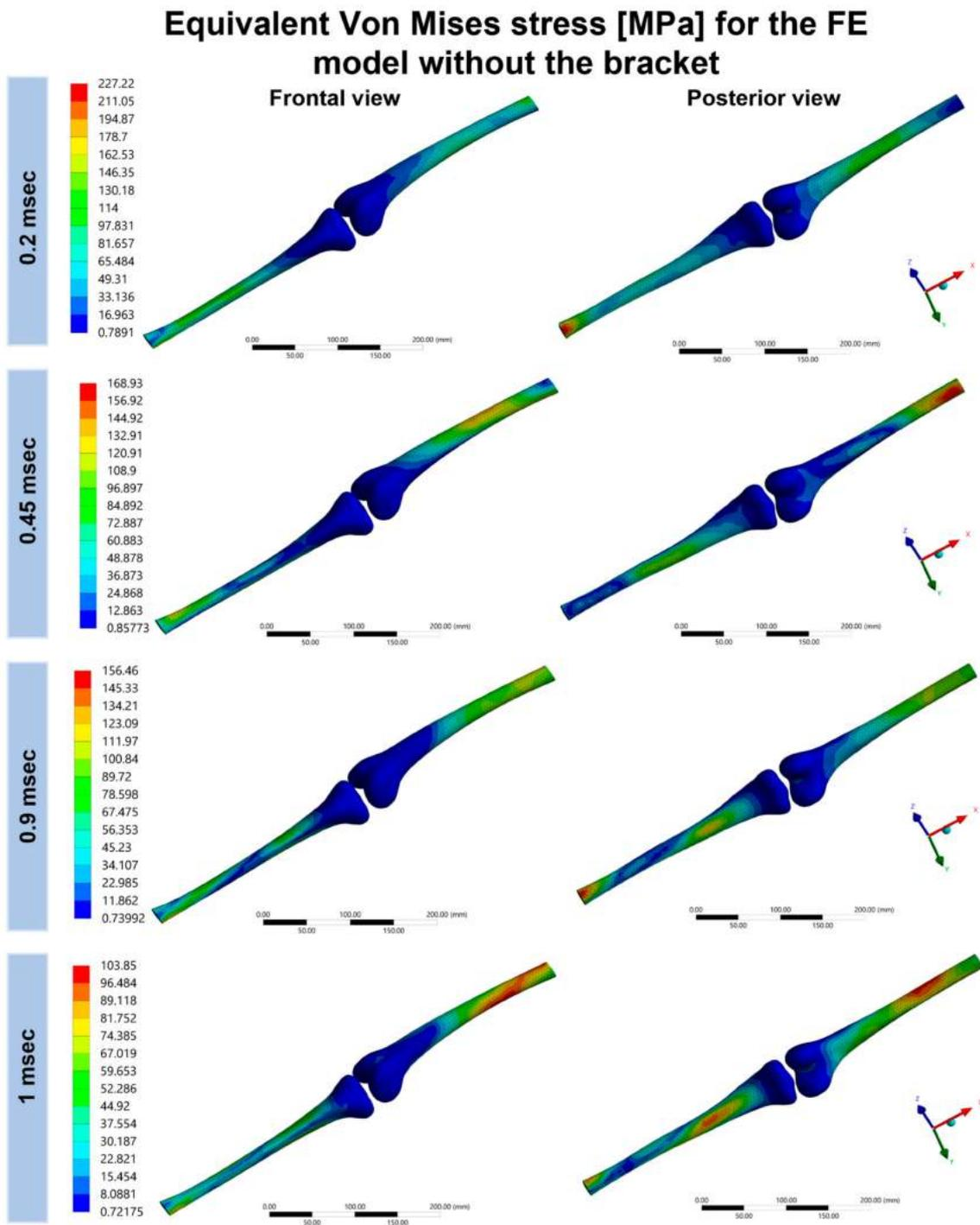
**Figure 9.** Equivalent Von Mises stress distribution in the bone component of the limb for the FE model without bracket.
