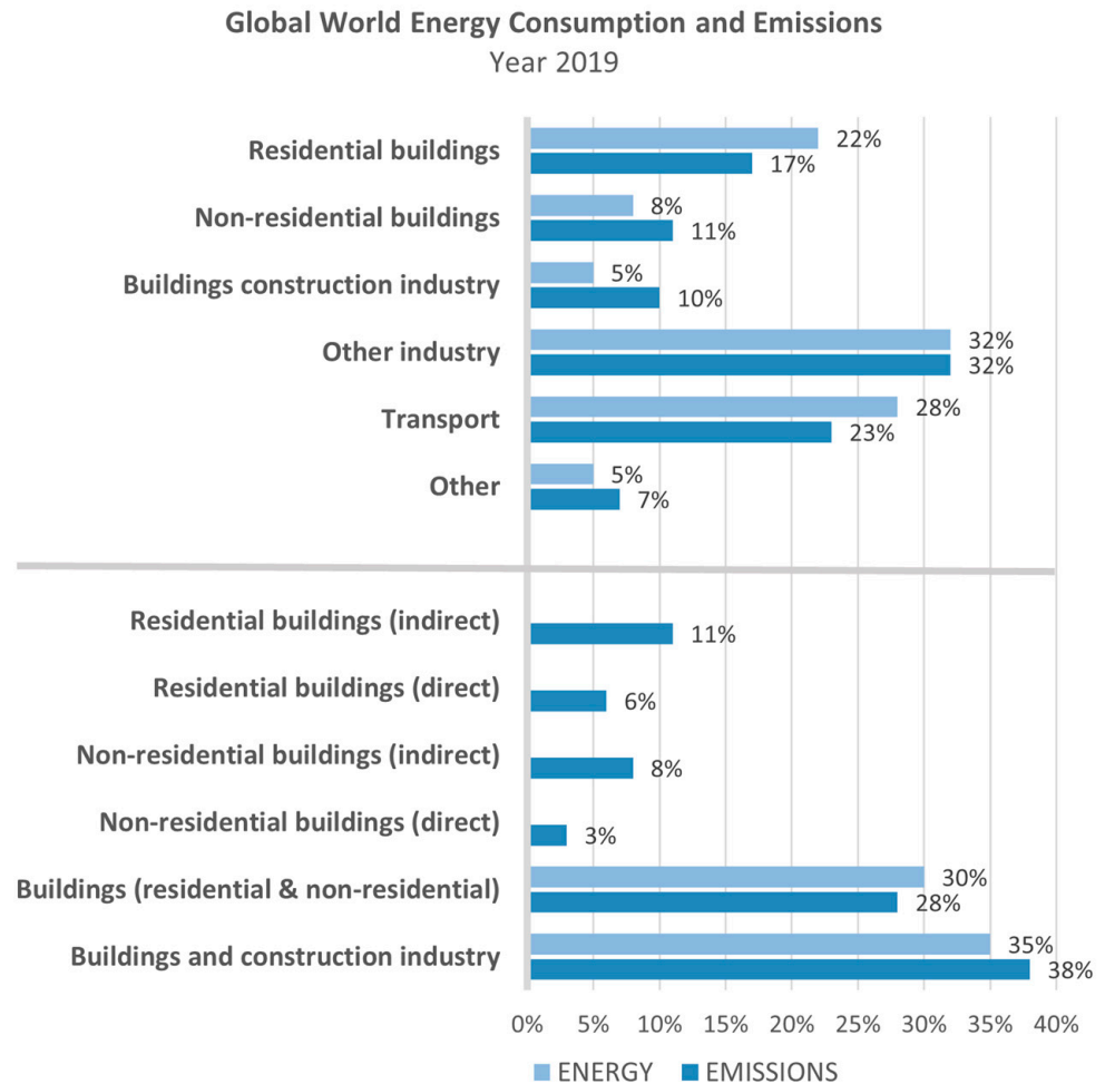
Figure 1. Global share of buildings and construction final energy and emissions, year 2019. Indirect emissions are emissions from power generation for electricity and commercial heat.
